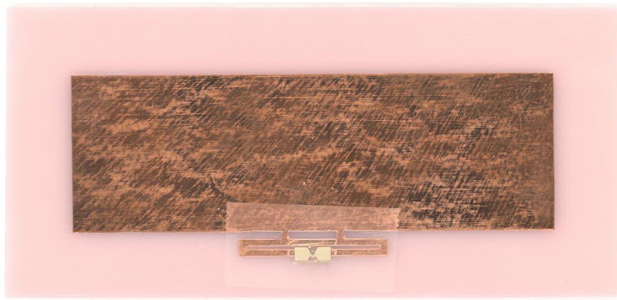
Figure 4.1a: Planar microstrip antenna with balanced feed mechanism – Prototype.
